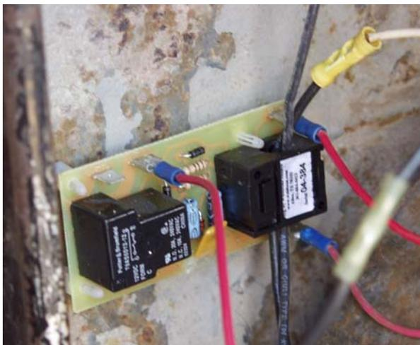
16. Mount the nylon standoffs on the panel by using the screws supplied. Once the standoffs are in place, simply push the circuit board over the standoffs until it pops in. Next, wire the electrical system for the control circuit board.
