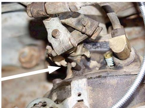
set correctly, **remove the jumper** from the oil pressure switch.
